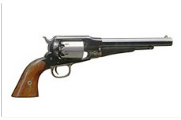
Remington Model 1858 percussion revolver, .36 or .44 caliber
