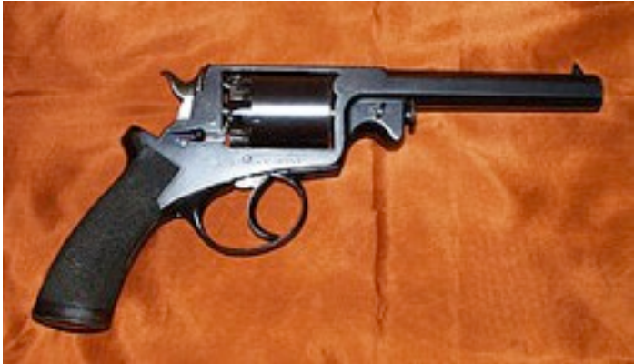
Beaumont-Adams, muzzle-loaded percussion revolver, .442 caliber, 54-bore, 11.2 mm
