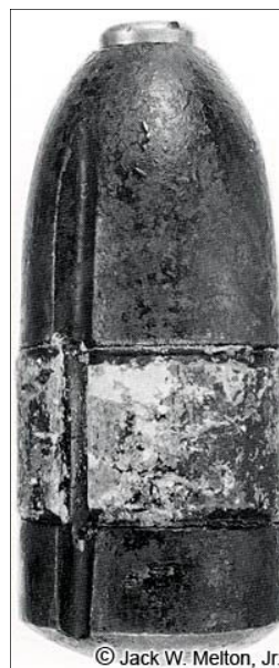
The Hotchkiss shell, the most common projectile fired from the Model 1861 3 inch rifled cannon. It was 2.94 inches in diameter, 6 and 7/8 inches long, and weighed 8.3 pounds. The Schenkl was another projectile fired from the same fieldpiece.
